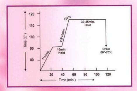
The goods are entered and run for 5 minutes. Predissolved Acrylic dye (with 98% gla. Acetic Acid), is added and the temperature of the bath is slowly raised to 90°c (1°c. / minute) 10 minutes hold at 90°c. Then the temperature of the bath is raised to 120° (0.5°c/minute). dyeing is continued for 30-45 minutes, depending on the depth of the shade. Bath is cooled to 60-70°c and drained, Goods are rainsed in cold and soaped at 80°c - 90°c.
